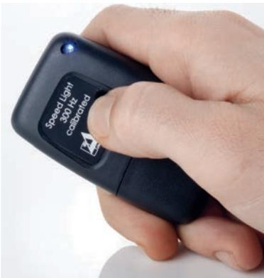
Press the button of the speed light and hold it over the scale so that it shines onto the strobe ring. The lines of the strobe ring indicating the chosen speed should appear to be stationary. If they are moving, then adjust the turntable speed according to the turntable user manual until the lines do not appear to move.
